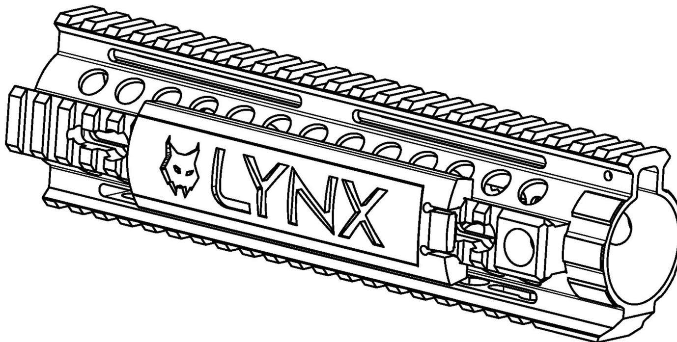
DUE TO THE DIFFERENT BRANDS, MODELS AND TOLERANCES, SOME PICATINNY RAILS CAN MAKE THE LTT FIT TOO TIGHT OR A BIT LOOSE.
